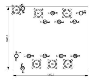
The third of the three tests, the service layout in the opening was carried out in accordance with annex F option 2:
